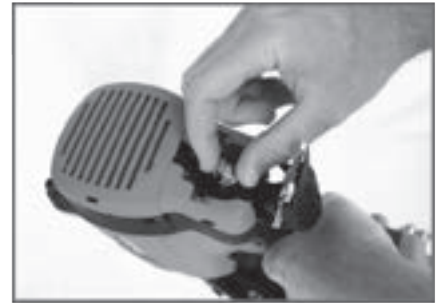
Carefully align fuel adaptor and cell stem
