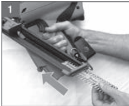
1 Slide nail strip into back of magazine
