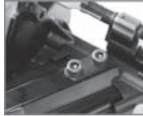
Remove 2 cap screws on side of magazine securing magazine to the nose
