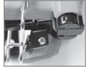
Remove nut from rear of magazine.
