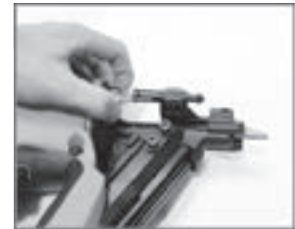
Reassemble tool, attach magazine to nose, replace cap screws and nut. Tool is ready to use.
