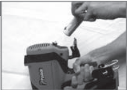
Raise fuel tube block assembly, it will lock in up position
