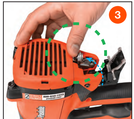
Lift fuel adapter to up position
