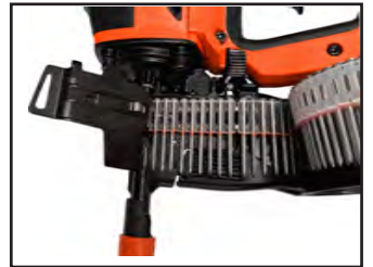
Insert nails into nose area
