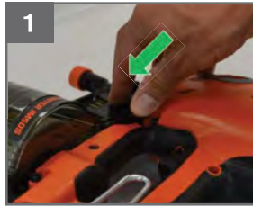
1 Push latch to open magazine gate
