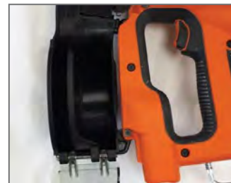
Swivel tray away from tool and slide to adjust for desired nail length
