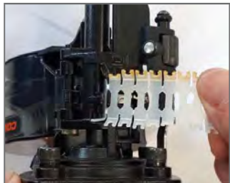
Fold tape at right angles across front of tool nose. Only then tear off collation
